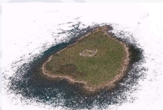
Surface model of the Croatian Island of Palacol derived from Structure from Motion (Image: Geert Verhoeven)
